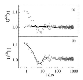
FIG. 2. Autocorrelation function for a 95 layer film (thickness 0.27  $\mu$ m) in the Sm-A phase at 50.1 °C. (a) Raw data (open dots) and reference signal from the NiC multilayer (filled dots). (b) Normalized correlation function obtained by dividing the raw data by the NiC reference signal; solid line is a fit to Eq. (1). For error bars, see text.
